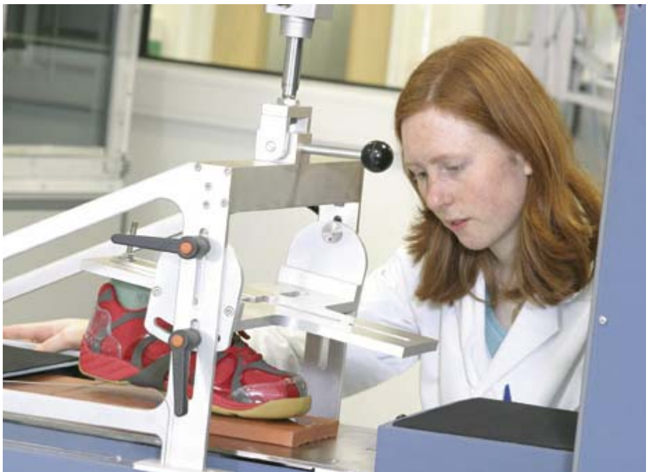
■ The SATRA STM603 slip rig provides customers with a knowledge of the slip resistance of floorings under a variety of conditions, usually to SATRA TM144:2004.
