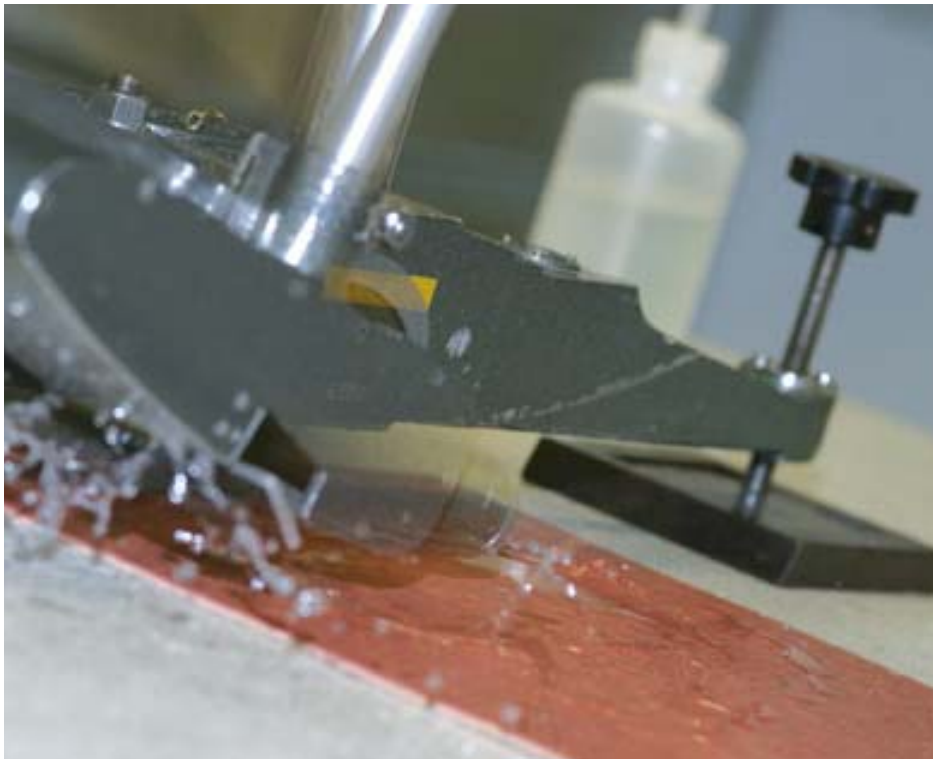
■ The BS 7976 Pendulum test is based on a swinging dummy heel. It sweeps over a specified area of flooring, just making contact with the surface.
